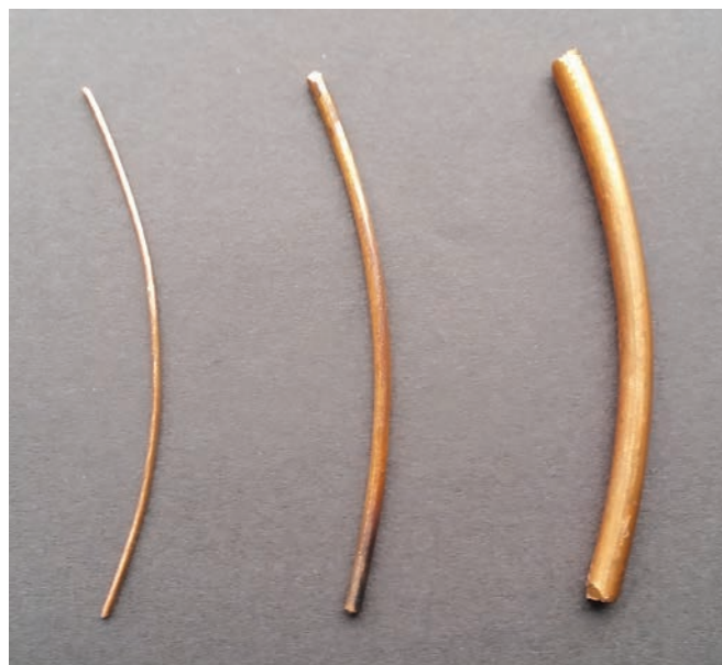
FIG. 5. Spacers for maintaining consistent HTC thickness. Shown left to right: \frac{1}{32} -in., \frac{3}{32} -in. and \frac{5}{32} -in. diameters.
